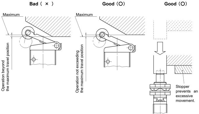
3. Operate the roller lever type from the following directions.
