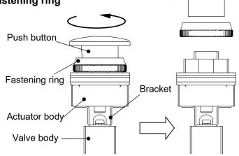
Remove the push button by holding the actuator body.
