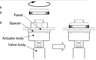
Mount the push button by holding the actuator body
