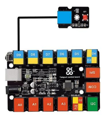
This module is compatible with the TS2178 TelePort control board.
