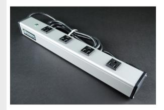
Four outlets, rugged gray aluminum housing, 15A, receptacles rotated 90 degrees and spaced to accommodate transformers. 15' [4.6m] 14/3 SJT black cord with NEMA5-15 plug. Length 16" [406mm]. Receptacle center-to-center 3" [76mm]. Snap-on, slide-off mounting.
