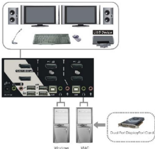
2. Use male-to-male DisplayPort video cable(s) to connect the DisplayPort connector(s) on the computer's video card, to one of the KVM's PC ports (i.e. PC1).
