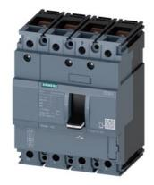
circuit breaker 3VA1 IEC frame 160 breaking capacity class N Icu=25kA @ 415V 4-pole, line protection TM210, FTFM, In=63A overload protection Ir=63A fixed short-circuit protection Ii=10 x In N conductor unprotected nut keeper kit
