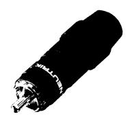
With PROFI, the ground before signal function is accomplished by a special shell element which protrudes - under spring load - out of the shell around the pin. It protects the pin from undesirable contacts with foreign potentials and provides a safe ground connection before the pin contact is closed.
