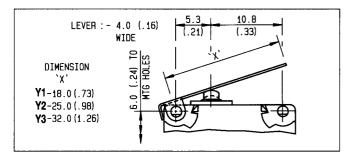
Y1, Y2, Y3 = Plain levers YR1 = Roller lever YC = Cam lever
