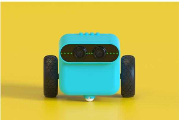
• While in its standby mode, press the power button to enter into the line-tracking & obstacles-avoidance mode, here lights on the LEDs in rainbow mode at the same time.
