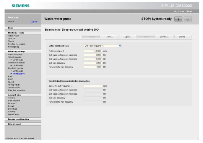
Image 10-28 Envelope spectra: Bearing types
