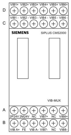
Image 8-2 VIB-MUX: Position of the connecting terminals
