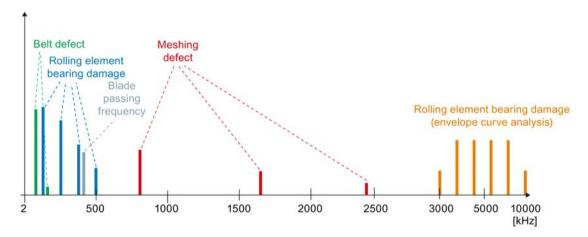
Image 3-6 Overall spectrum of vibration acceleration
