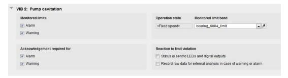
Image 10-25 Envelope spectra: VIB channel with fixed speed
