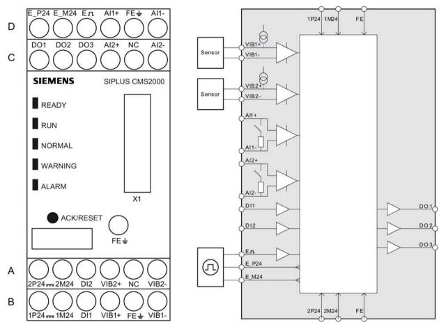
Image 8-1 Terminal assignment and block diagram
