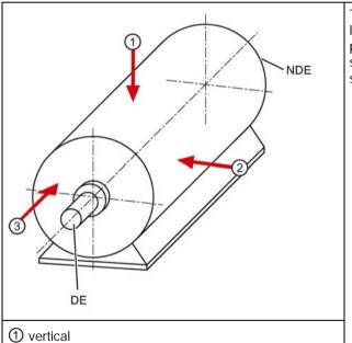
The measurements are taken at the installation site of the machine. The standard provides information about the choice of suitable measuring points for the vibration sensors.
