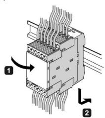
Image 7-1 Mounting of Basic Unit VIB
