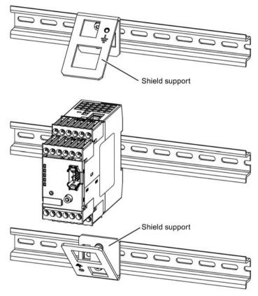
Image 7-2 Mounting the shield support
