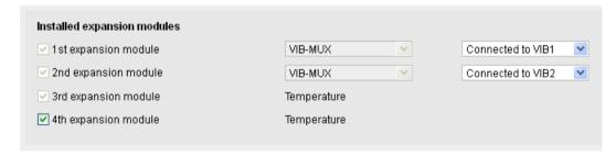
Image 10-46 Installed expansion modules (VIB-MUX and temperature modules)
