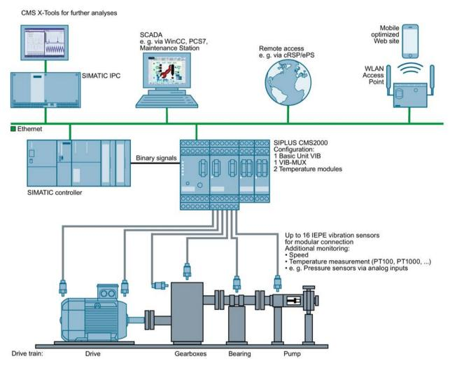
Image 4-3 Integration into system environments
