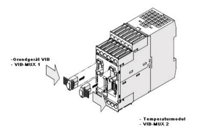
Image 8-3 Expansion module: Connection via system interface
