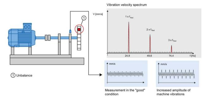
Image 3-5 Example of a spectrum of vibration velocity (unbalance)
