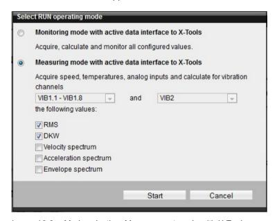
Image 10-3 Mode selection: Measurement mode with X-Tools
