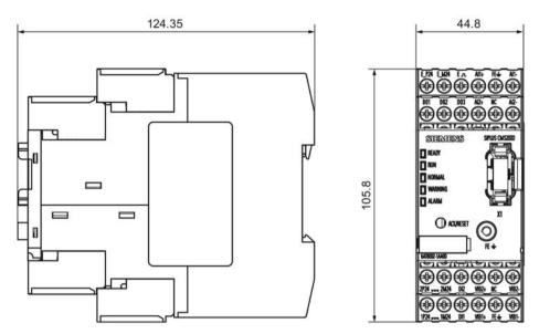
Image 13-1 Dimension drawing SIPLUS CMS2000 Basic Unit VIB
