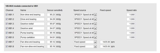
Image 10-52 VIB-MUX module connected to VIB1/2
