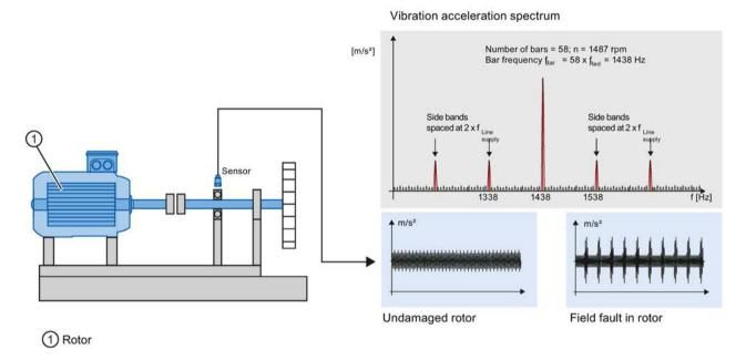
Image 3-7 Example: Spectrum of the vibration acceleration (rotor field fault)
