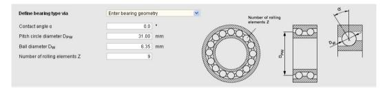
Image 10-30 Defining the bearing type by entering the bearing geometry
