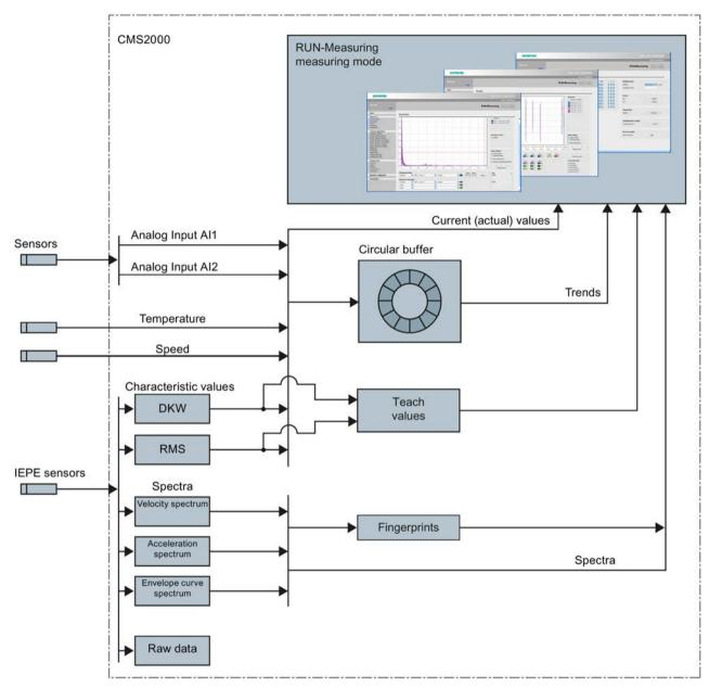
Image 5-2 Measurement mode method of operation
