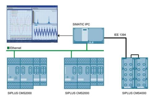
Image 5-4 Typical system configuration
