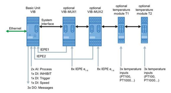
Image 4-2 System configuration CMS2000 maximum configuration
