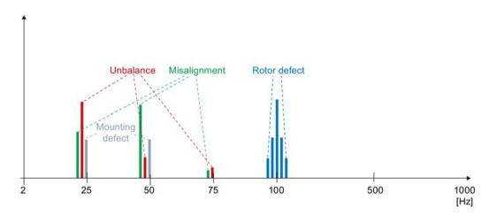
Image 3-4 Overall spectrum of vibration velocity
