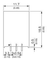
Dimensions in mm (inch) Tolerances: x.x  $\pm 0.5$  ( $\pm 0.02$ )  $x.xx \pm 0.25 (\pm 0.01)$ Pin dimension tolerance ±0.004 (±0.1)
