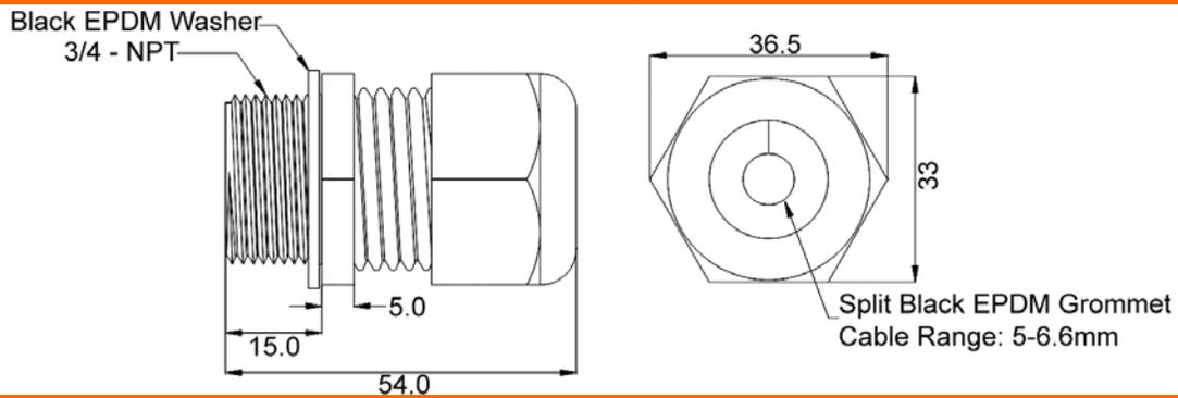
Double Cable Gland - PGLAND750-2\* Dimension Diagram unit:mm
