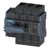
Switch disconnector 125 A, Size 2, 3-pole Front operating mechanism left Complete unit with direct operating mechanism gray Box terminal
