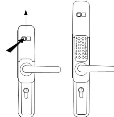
**9** Enter the code in place, then lower the handle : the spring bolt retracts, allowing the door to be opened.
