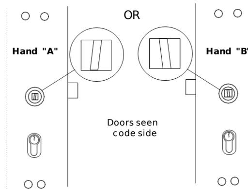
**5** Assemble the front panel (if necessary: change the combination and / or modify the permanently-open option beforehand) (see other instructions)
