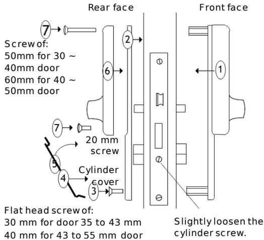
**7** Immediately check that the inner handle drives the spring bolt without any difficulty.
