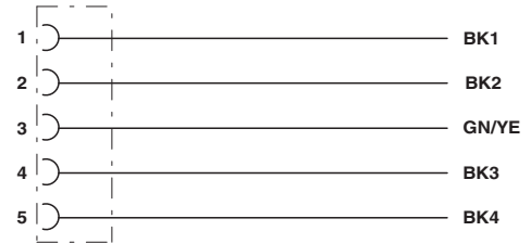
Contact assignment of 7/8" socket
