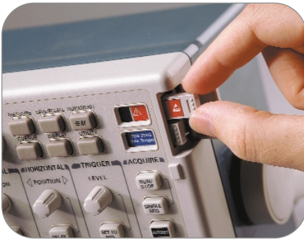
► Application module being installed.
