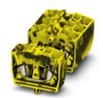
Mini feed-through terminal block, Connection method: Spring-cage connection, Cross section: 0.08 mm² - 4 mm², AWG: 28 - 12, Width: 10.4 mm, Height: 22 mm, Color: black/yellow, Mounting type: On mounting plate
