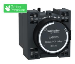
Time delay auxiliary contact block, TeSys Deca, 1NO + 1NC, off delay 0.3-3s, front, spring terminals
