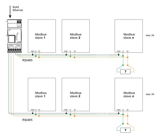
Fig. 3 Modbus RTU connection. COM 1 master, COM 2 master
