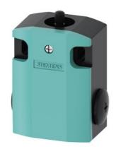
Basic switch for position switch 3SE5112 Metal enclosure 56 mm 3x (M20x 1.5) 2 NO/1 NC slow-action contacts without actuator head
