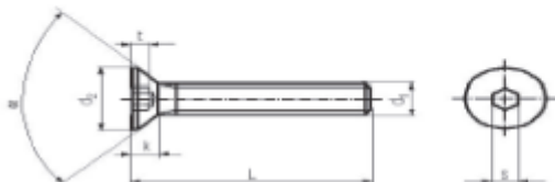
FLAT HEAD SOCKET CAP SCREWS DIN 7991 / ISO 10842 / ANSI B18.3.5M
