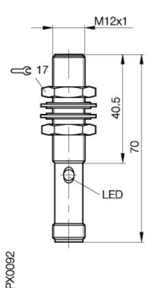
**Inductive Sensors** BES 516-370-S 4-C M12x1 x 70 normally-closed Sn=2mm shielded
