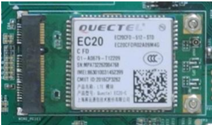
Figure 17: mini-PCIe Connector&4G Module
