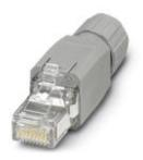
RJ45 connector, degree of protection: IP20, number of positions: 8, 1 Gbps, CAT5 (IEC 11801:2002), material: PA, connection method: IDC fast connection, connection cross section: AWG 26-23, cable outlet: straight, color: traffic grey A RAL 7042
