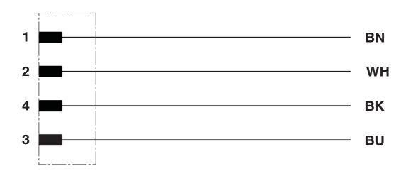
Contact assignment of the M12 plug
