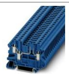
Disconnect terminal block, Connection type: Screw connection, Cross section: 0.14 mm² - 6 mm², AWG: 26 - 10, Nominal current: 20 A, Nominal voltage: 500 V, Length: 65.4 mm, Width: 6.2 mm, Color: blue, Assembly: NS 35/7,5, NS 35/15
