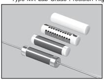
Non-Inductive serpentine pattern with a patented, high thru-put screen printed silicone coating. The alignment of the gap in the coating pattern with the gap in the serpentine resistor pattern provides a complete encapsulation of the resistor element. The cap and lead assemblies are pressed onto the resistor core, finishing the resistor and providing rugged terminal attachment.
