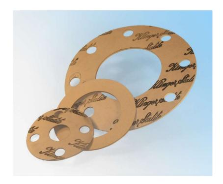
KLINGERstatite is an impregnated paper gasket providing reliable sealing at low cost for applications where the additional strength offered by fibre reinforcements such as aramid, glass or carbon is not a requirement. Paper-based materials are often used in low-temperature and low-pressure applications.
