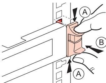
The quick fixing for metal panels is compatible with 1.4 to 2.75 mm thick 19" uprights with 8.25 to 9.5 mm square perforations. An automatic equipotential link is ensured with 19" LCS<sup>2</sup> uprights. Direct clipping on of plastic panels is compatible with 1.5 to 2 mm thick 19" uprights with 9.5 mm square perforations.
