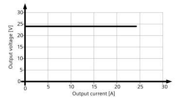
Figure 6-6 Output characteristic 6EP3336-3SB00-0AX0 (24 V/20 A)
