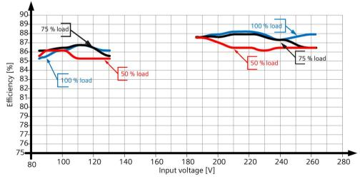
Figure 6-8 Efficiency 6EP3333-3SB00-0AX0 (24 V/5 A)
