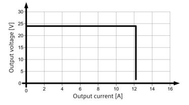
Figure 6-5 Output characteristic 6EP3334-3SB00-0AX0 (24 V/10 A)
