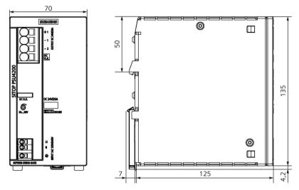
Figure 2-9 Dimension drawing 6EP3336-3SB00-0AX0 (24 V/20 A)
