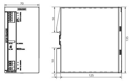
Figure 2-8 Dimension drawing 6EP3334-3SB00-0AX0 (24 V/10 A)
