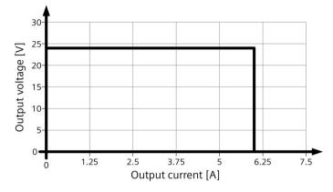
Figure 6-4 Output characteristic 6EP3333-3SB00-0AX0 (24 V/5 A)
