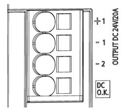
Figure 5-2 Connecting the output voltage (example 6EP3336-3SB00-0AX0)
