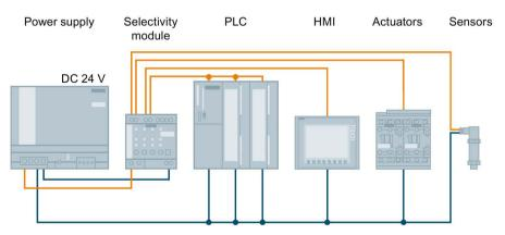
Figure 9-5 Electronic protection of 24 V loads using the SITOP PSE200U selectivity module
