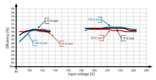
Figure 6-9 Efficiency 6EP3334-3SB00-0AX0 (24 V/10 A)
