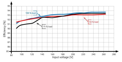
Figure 6-10 Efficiency 6EP3336-3SB00-0AX0 (24 V/20 A)
