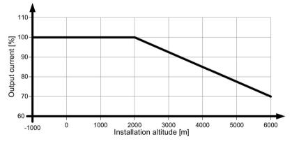
Figure 4-5 Mounting height derating
