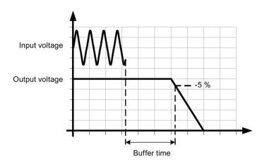
Figure 6-1 Power failure buffering
