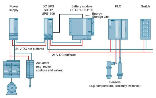
Figure 9-8 24 V buffering with SITOP UPS1600 to maintain communication, signaling functions, sensor measured values and position values
