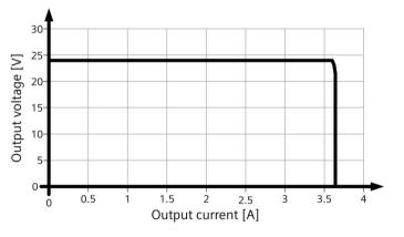
Figure 6-3 Output characteristic 6EP3332-3SB00-0AX0 (24 V/3 A)
