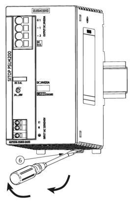
Figure 3-1 Mounting/removal (example 6EP3336-3SB00-0AX0)
