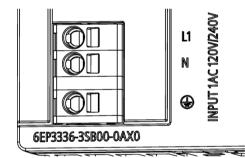
Figure 5-1 Line connection (example 6EP3336-3SB00-0AX0)
