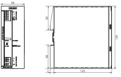
Figure 2-7 Dimension drawing 6EP3332-3SB00-0AX0 (24 V/3 A) and 6EP3333-3SB00-0AX0 (24 V/5 A)
