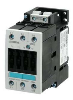
CONTACTOR, AC-3 22 KW/400 V, AC 110V 50HZ/120V 60HZ 3-POLE, SIZE S2, SCREW CONNECTION
