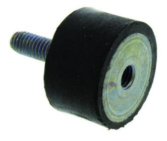
Their elasticity is much greater in all the directions parallel to the armatures than in the perpendicular direction. The rubber works based on compression or shear depending on the direction it is placed in at installation time. This direction is made according to the use and the objective.
