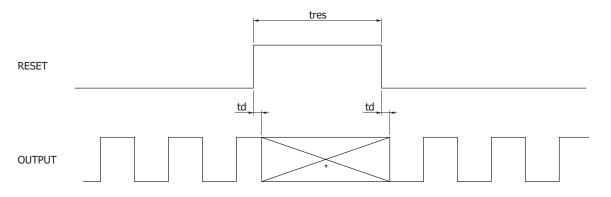
\* OUTPUT terminal is at High impedance during RESET period ("High" state).
