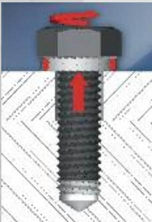
**An important feature of HEICO-LOCK wedge lock washers, setting them apart from other systems that are available, is the securing of the bolt fastening using preload force rather than friction**
