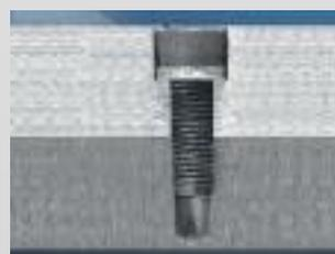
Countersunk secured cylinder bolt
