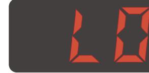
Low temperature alarm (AL, Ad & A0 parameters)
