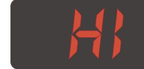
High temperature alarm (AH, Ad & A0 parameters)
