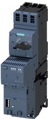
intelligent load feeder direct starter high feature 0.4-4 A up to 690 V AC type of coordination 2 frame size S00 for ET 200SP system consisting of 3RC7140-1EE10, 3RV2311-1EC20, 3RT2017-2BB42
