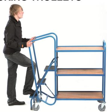
These Order Picking Trolleys have sprung loaded steps with ribbed rubber on plywood treads set into rolled steel angle frames.
