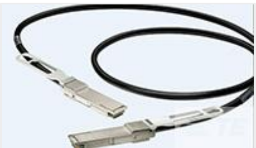
TE Part # 2829040-8 QSFP IB EDR, 26AWG, 3.0M
