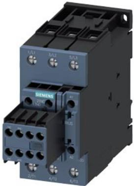
power contactor, AC-3e/AC-3, 65 A, 30 kW / 400 V, 3-pole, 48-80 V AC/DC, 50/60 Hz, with integrated varistor, auxiliary contacts: 2 NO + 2 NC, screw terminal, size: S2, removable auxiliary switch
