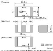
\*1 There is no electrical polarity, but there is a directional marking on the top of the product to identify inner physical direction.
