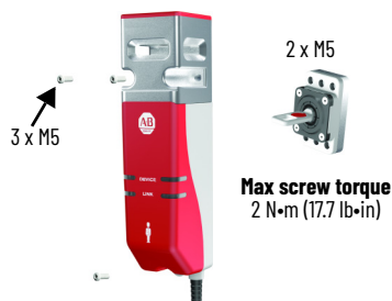
Figure 2 - Required Mounting Hardware for Switch and Actuator
