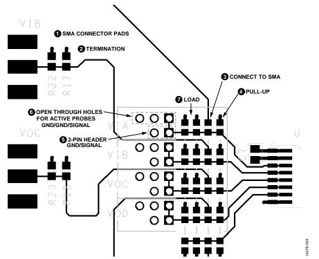
Figure 4. Configuration and Monitoring Structures (Showing a Datapath from an External Connection to the DUT Pin)
