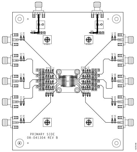
Figure 6. Top Level Signal Routing and Assembly
