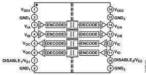
Figure 2. Functional Block Diagram of the ADuM140D/ADuM140E
