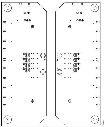
Figure 7. GND1 and GND2 Planes
