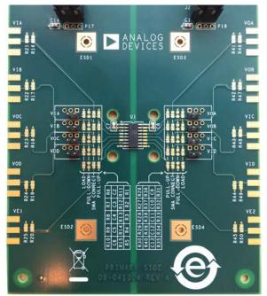
Figure 1. EVAL-3CH4CHSOICEBZ Evaluation Board with the iCoupler Digital Isolator Installed
