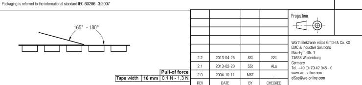
DESCRIPTION **WE-PD SMD Shielded Power Inductor** COMPLIANT SIZE 744777127 A4 Size: 7345
