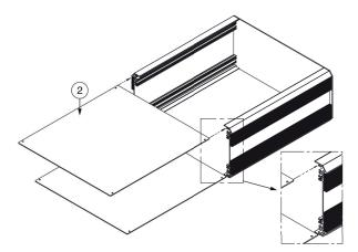
3. Slide the ② top/bottom covers into the side frame slots.
