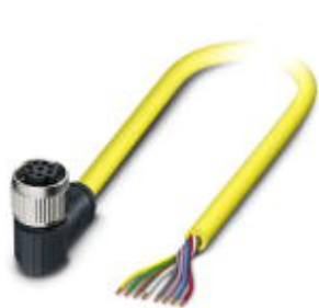
Sensor/Actuator cable, 8-position, PVC, yellow, Free cable end, on Socket angled M12 SPEEDCON, A-coded, Cable length: 2 m
