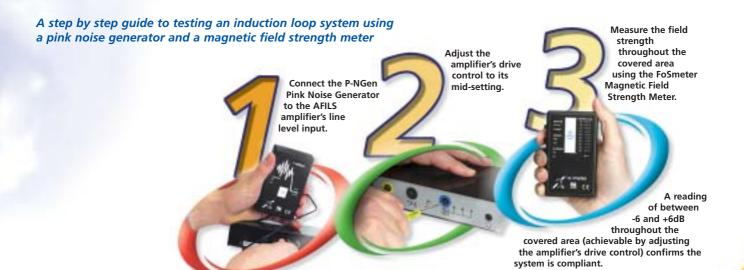
Important: Once you have verified the magnetic field strength of the system, we recommend you listen to the system's real audio source(s) using a loop listening device (such as the FoSmeter H) to ensure there is no 'clipping' or distortion. If any adjustments need to be made to the amplifier's settings, be sure to re-test the system using the P-NGen pink noise generator and a FoSmeter variant before signing the installation off.
