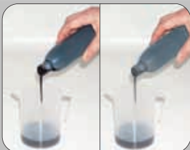
1. Pour the 2 components in equal quantity in the becker
