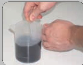
2. Mix the poured components in the becker (30" max)
