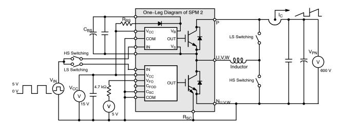
Figure 5. Example Circuit for Switching Test
