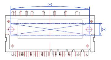
Figure 9. Flatness Measurement Position
