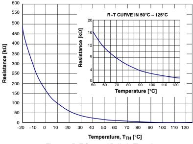
Figure 7. R-T Curve of Built-in Thermistor
