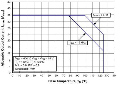
Figure 8. Allowable Maximum Output Current
