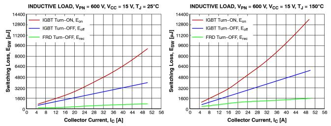
Figure 6. Switching Loss Characteristics (Typical)
