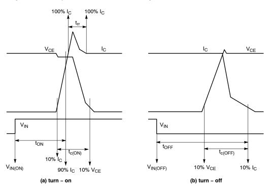
Figure 4. Switching Time Definition
