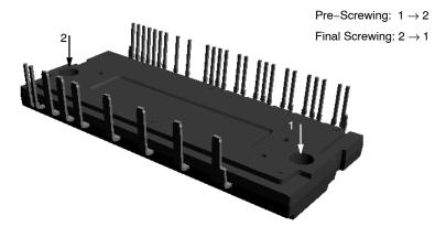
Figure 10. Mounting Screws Torque Order
