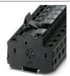
Fuse modular terminal block, Connection method: Screw connection, Cross section: 1.5 mm²- 25 mm², AWG: 16 - 4, Nominal current: 32 A, Nominal voltage: 690 V, Width: 18 mm, Fuse type: Midget / 10.3 x 38, Fuse type: Glass, Mounting type: NS 35/7,5, NS 35/15, Color: black
