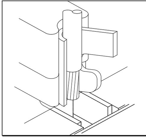
8. Keeping the cable steady in the crimp, fully close the hand crimp tool until the ratchet releases. Let the crimp tool open.
