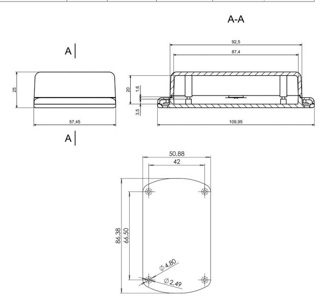
Dashed line shows outline of the mounting elements under PCB board All dimensions are given within +/-0,25mm tolerance
